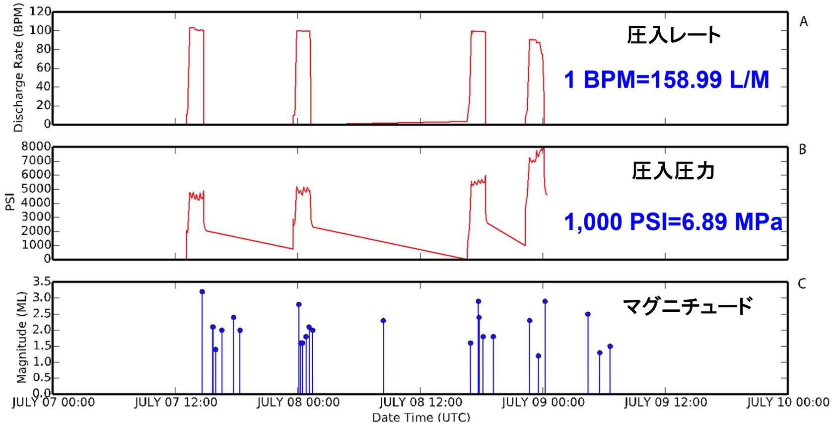
Figure 4. The plots span, in UTC time, the four fracking stages of Eagleton 1-29 well between July 7<sup>th</sup> 2014 and July 9<sup>th</sup> 2014. Plot A shows the discharge rate in BPM, or rate of injection, through time, plot B shows the pressure in PSI through time and plot C shows magnitude of earthquakes occurring within 7.0 km of the Eagleton well through time.
