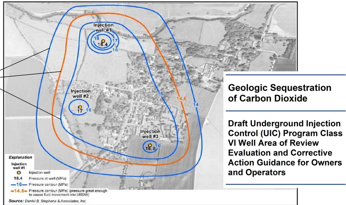
Figure 3-3: Hypothetical Geologic Sequestration Site: Model Predicted Maximum Pressure Within the Injection Zone
