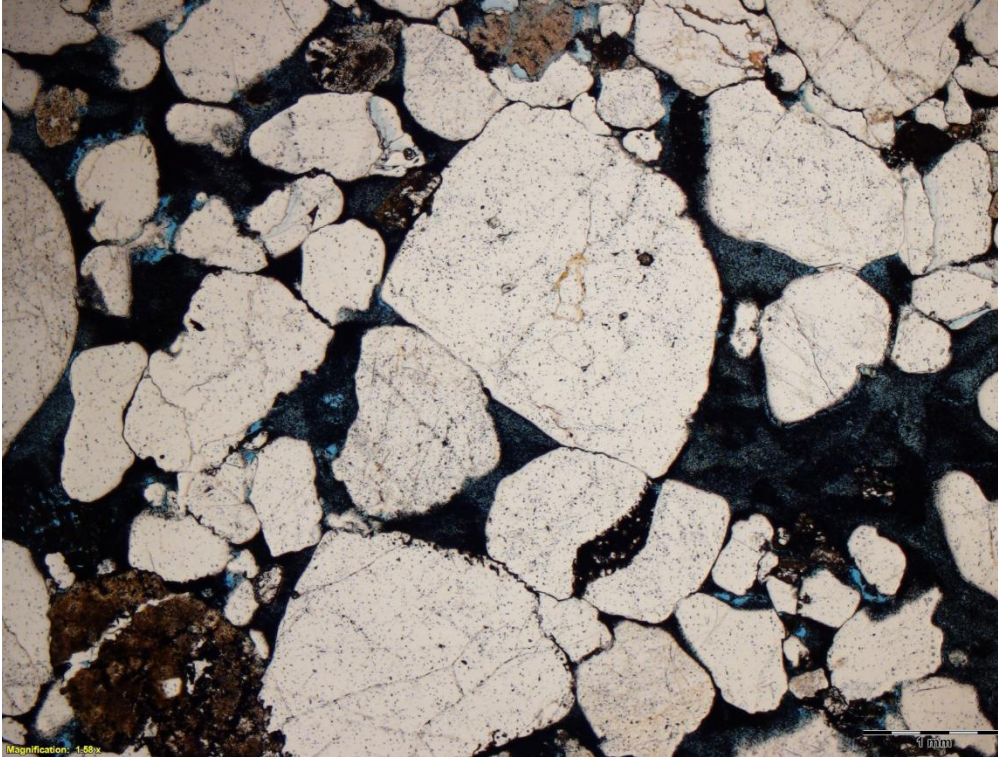
Poorly sorted grains with abundant pore filling clay
