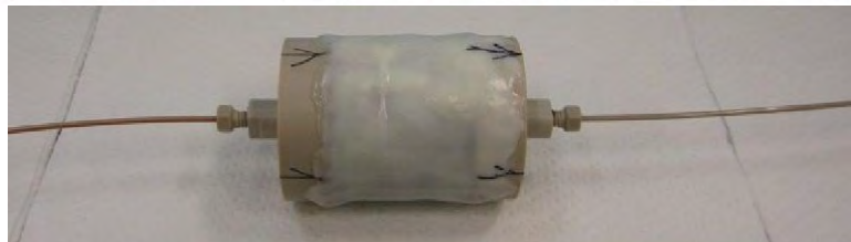
Sandstone prepared for Super-critical CO 2 injection (10 MPa, 40°C)
