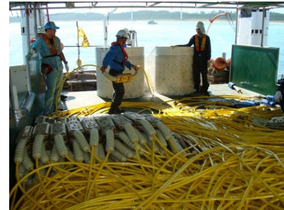
OBC cable deployment (by JGI)
