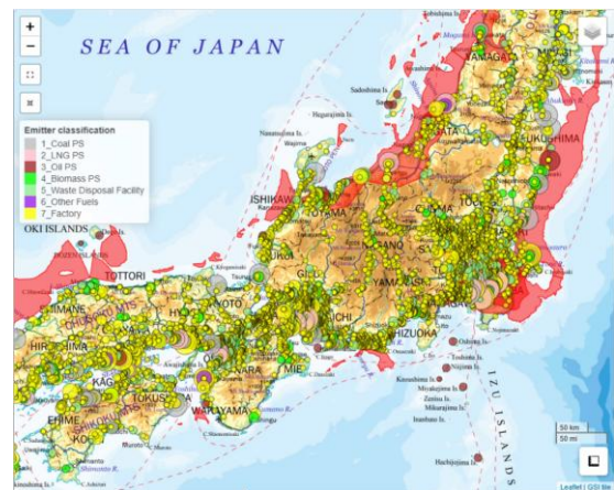
Figure 9: Spatial mapping of major CO 2 emission sources and potential geological storage sites across Japan, integrated into the CO 2 Emission Source Database.
