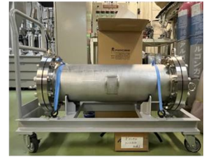
Membrane module ( \phi = 20 cm; L = 60 cm)
