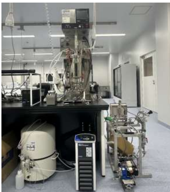
5 L Jar fermenter - membrane separation system
