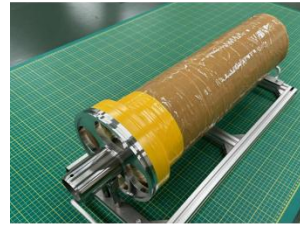
Membrane element ( \phi = 20 cm; L = 60 cm)
