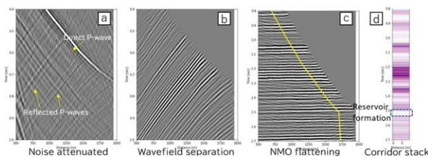
Figure 5 DAS/VSP recording and data processing examples
