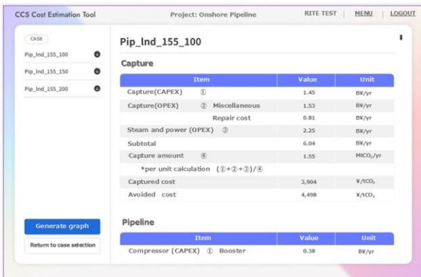
Figure 13 Output screen of the calculation results (table)
