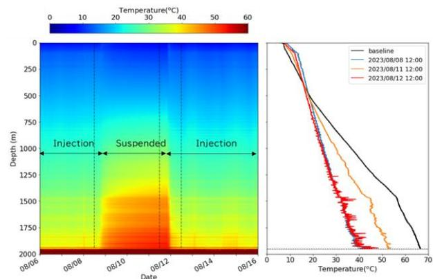
Figure 6 Example of injection monitoring using DTS
