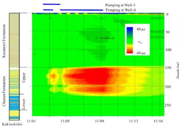
Figure 3 DSS measurement example at Mobarate site
