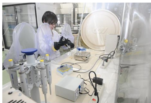
Fig.6 Anaerobic chamber for genetic manipulation
