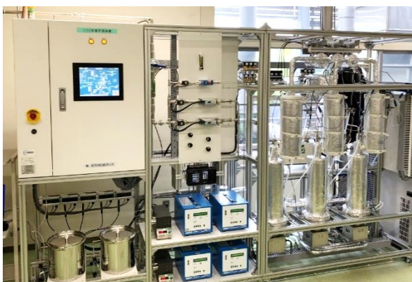
Fig. 12 Lab test equipment for DAC
