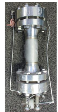
Membrane module (2-inch)
