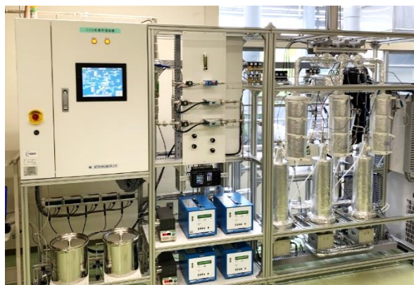
Fig. 8 New designed lab test equipment for DAC
