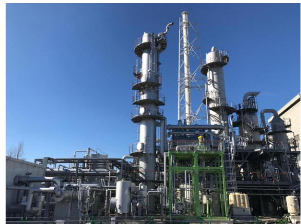
Fig. 1 Equipment of energy-saving CO 2 absorption process ESCAP ® at Niihama Nishi power station, Sumitomo Joint Electric Power Co., Ltd.
