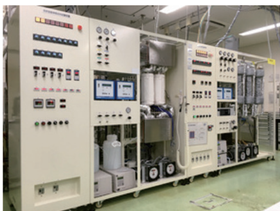
Fig. 6 : Lab-scale fixed-bed apparatus for CO 2 capture test
