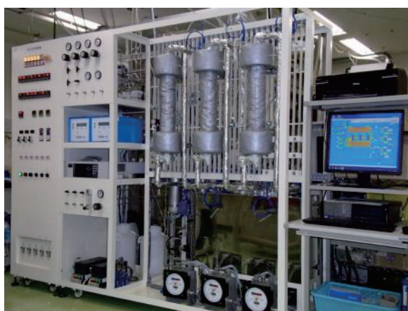
Fig. 7 : Lab-scale apparatus for CO 2 capture test
