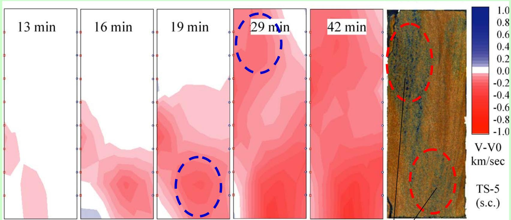
*CO<sub>2</sub> flows parallel to bedding plane; Numeric numbers: Elapsed time*
