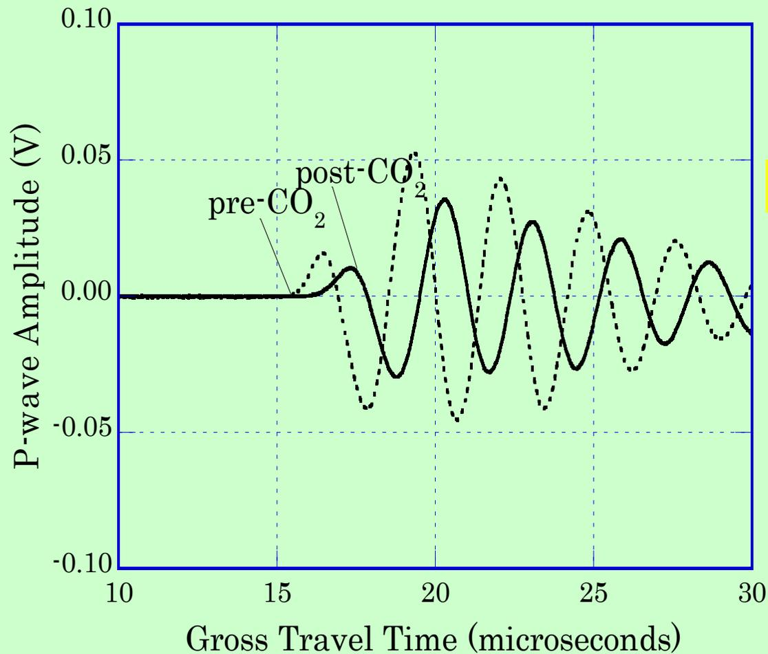
*P-wave forms obtained from pre- and post- CO<sub>2</sub> flooding in Tako sandstone.*
