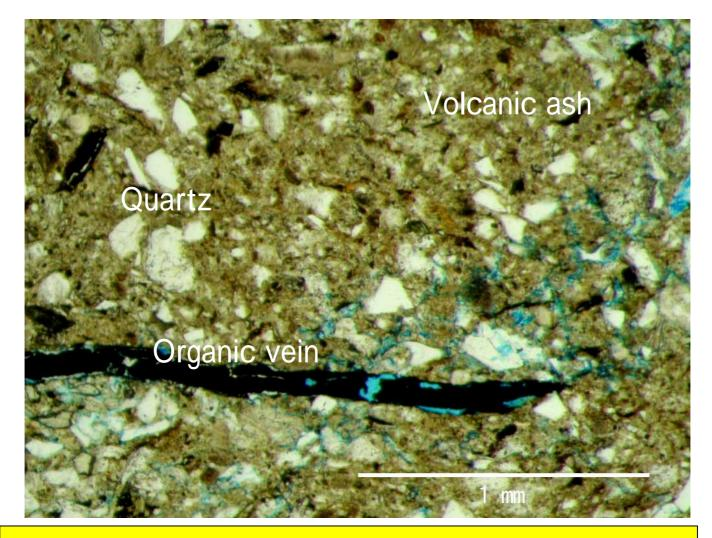
Siltstone as caprock of Nagaoka injection test site
