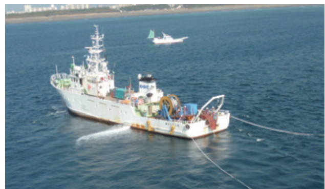
Figure 6 Laying permanent OBC observation system
