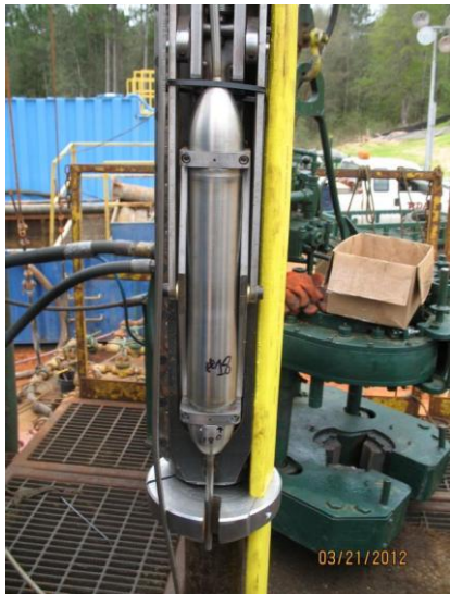
Geophone in clamp with flatpack
