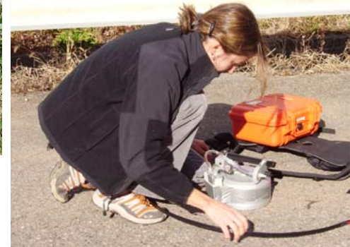
Flux accumulation chamber
