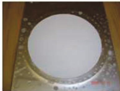
20 cm 2 lab-scale flat-sheet
