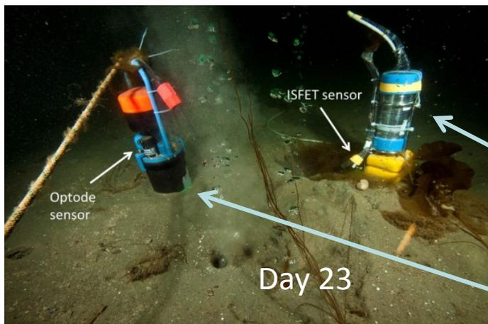
Measuring CO<sub>2</sub> via pH/pCO<sub>2</sub> can be very dependent on sensor positioning:
