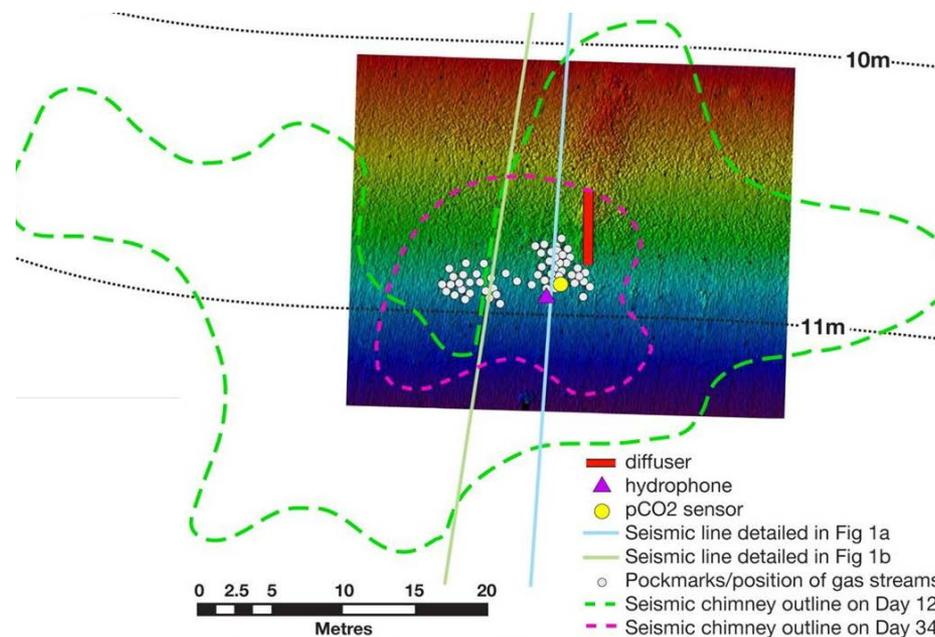
Seismic reflectance can “see” gas above a threshold. Flow mechanisms are complex
