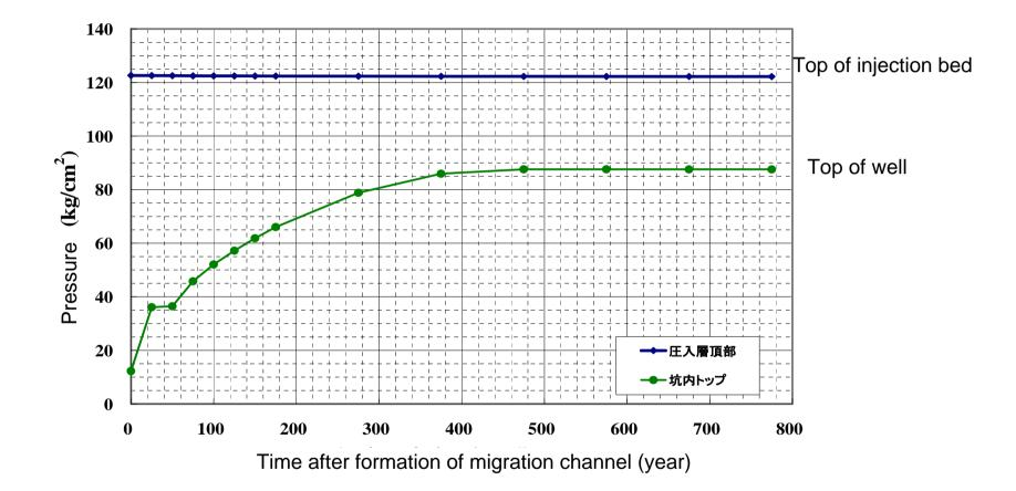
Permeability of cement plug 1,000 md, Permeability of crack 10,000 md, Area ratio of crack 10% Simulation software GEM-GHG
