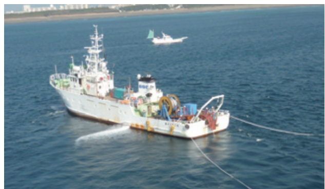
Figure 6 Laying permanent OBC observation system
